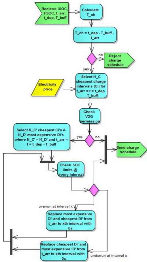
Fig. 7. EV charging algorithm flowchart.
