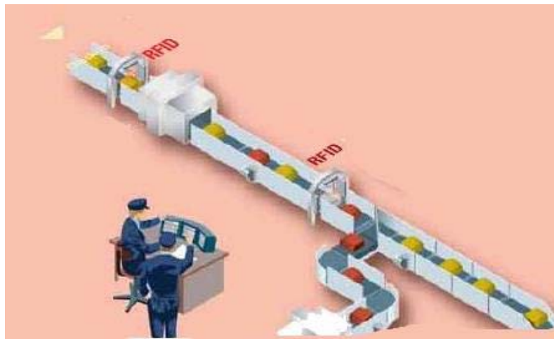
Figure 5. RFID readers in baggage handling stations
